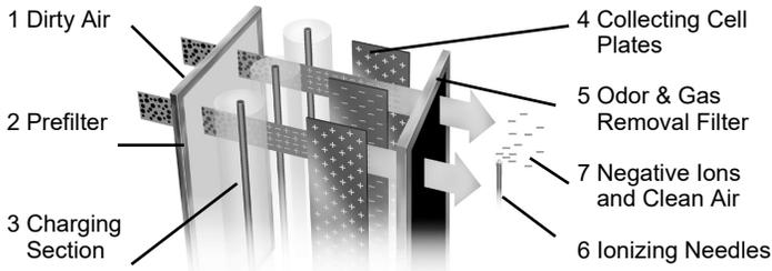
Dirty air is drawn in through the front grill and passes through a 4-stage filtering system.
